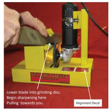
Picture demonstrates the angle and method to sharpen.
